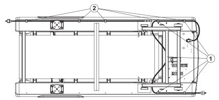
Note: It may be necessary to tip the treadmill to route the power cord properly.
